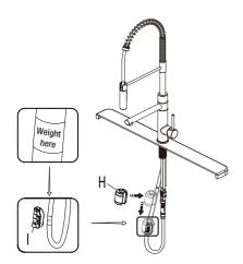
Install the weight clip (I) at the point of the hose marking "weight here". Insert the weight (H) onto the weight clip (I) by sliding it down onto the weight clip (I).
