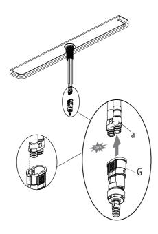
Push the 3-way quick connect assembly (G) firmly upward and attach it to the receiving block (a). Pull down moderately to ensure the connection has been made.
