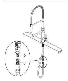
Push the quick connector (J) firmly upward and attach it to the receiving block (b). Pull down moderately to ensure the connection has been made.
