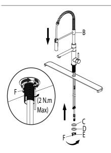
Shut off the water supply. Place faucet (B) through the hole in countertop. Secure the faucet (B) to the countertop using the rubber washer (C), metal washer (D) and mounting nut (E) provided. Tighten screws (F).
