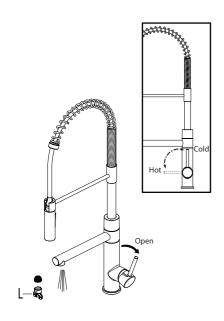
Important: After installation is complete, remove aerator with aerator key (L). Turn on water supply and allow both hot and cold water to run for at least one minute each. While water is running, check for leaks. Replace aerator. This flushes away any debris that could cause damage to internal parts.
